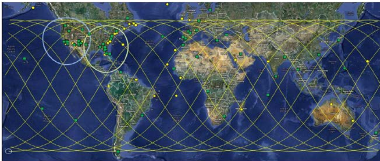
Figure 2. Dream Chaser Landing Opportunities. Extensive cross-range capability of more than 1,100 nmi (distance illustrated by circles) allows for frequent landing opportunities on every CONUS overflight. The dots (yellow and green) indicate possible Dream Chaser landing and abort locations for an ISS mission, while the yellow dots indicate previous shuttle landing and abort locations.
