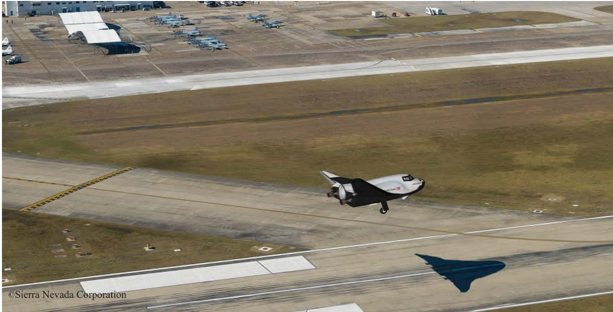
Figure 3. Artist Concept of Dream Chaser Landing at Ellington Airfield, Houston, Texas. The Dream Chaser vehicle can land at any suitable runway that is at least 8,000 feet long.
