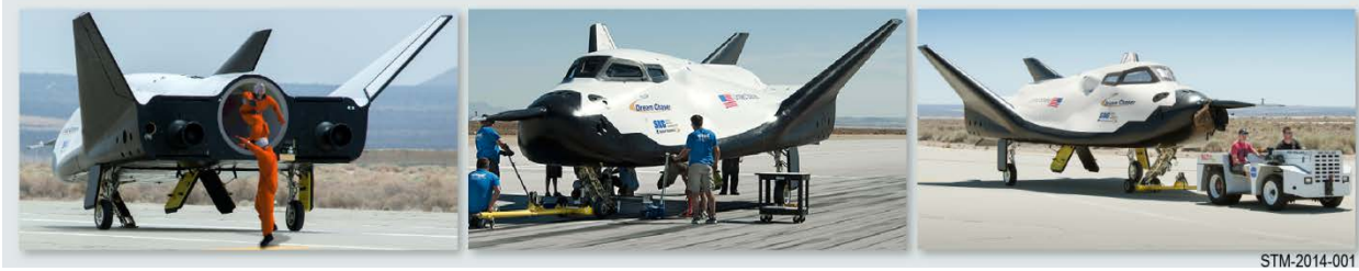
Figure 10. Dream Chaser Removal from Runway and Crew Egress. The Dream Chaser's design allows unassisted crew egress at any landing site without the need for special equipment. This operation nominally occurs after the vehicle has been towed off the runway. The minimum equipment needed to quickly remove the vehicle from the runway is enabled by the low toxicity and low hazard levels of the Dream Chaser design, thus minimizing the impact on day-to-day operations at a public-use landing site.
