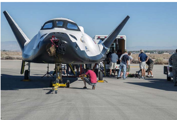
Figure 11. Dream Chaser Attachment to Ground Support Equipment. The Dream Chaser design allows for standard ground support equipment (tow bar and cooling cart) to interface with the vehicle after removal from an active runway.
